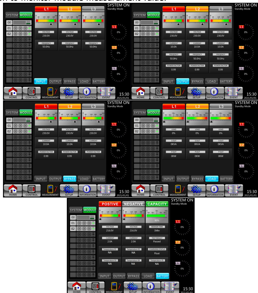
Figure 4-10 Module Measurement Screens
