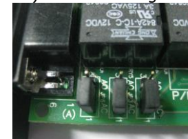
Fig. 6 Jumper setting for ACTIVE CLOSE
